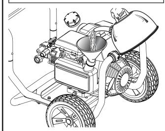
This is a 4-cycle engine. Do not mix fuel and lubricant together.
