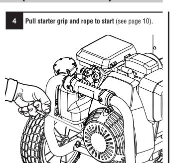
Allow engine to run for several seconds, then move choke to RUN position (see page 10).
